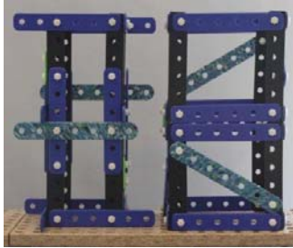
Figure 1a: High Alignment condition: stable (braced) model on left, unstable model on right
