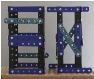
Figure 1b: Low Alignment condition: unstable model on left, stable (braced) model on right, showing the two counterbalanced versions
